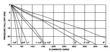
Note: Flow curves are based on static conditions of 100 psi inlet pressure and 50 psi outlet pressure. Pressure Fall-off is the decrease in downstream regulated pressure when the flow increases.
